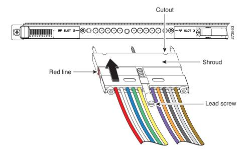
Figure 18 Installing the UCH on the Faceplate
